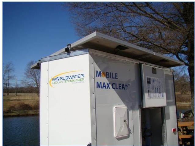
720 watts integrated onto trailer
