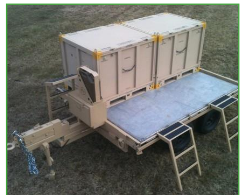
Trailer deployed with 463L pallet and JMIC containers
