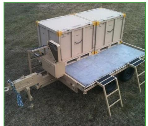
Trailer deployed with 463L pallet and JMIC containers
